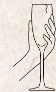
Remove damaged or abraded glassware from service (damaged glass may break in the dishwasher).
